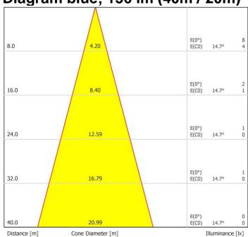
Distance [m] Cone Diameter [r C0 - C180 (Half-value Angle: 29.4°)
