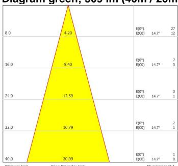
Distance [m] Cone Diameter [m] Co - C180 (Half-value Angle: 29.4°)
