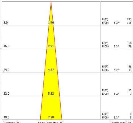
Distance [m] Cone Diameter [m] C0 - C180 (Half-value Angle: 10.4°)
