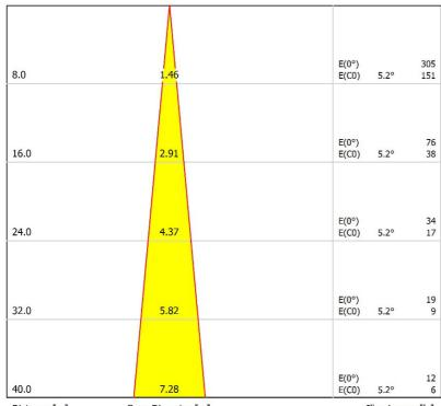
Distance [m] Cone Diameter [m] Co - C180 (Half-value Angle: 10.4°)
