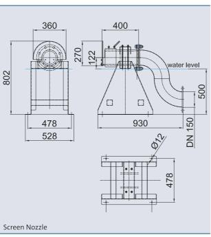
The nozzle creates a filmy water screen. This qualifies for projection of Laser, Video, Slide and Gobo (Graphical optical blackout) type of illumination. Based on the law of physics of light, the position of the nozzle should always be between the viewer and projector.
